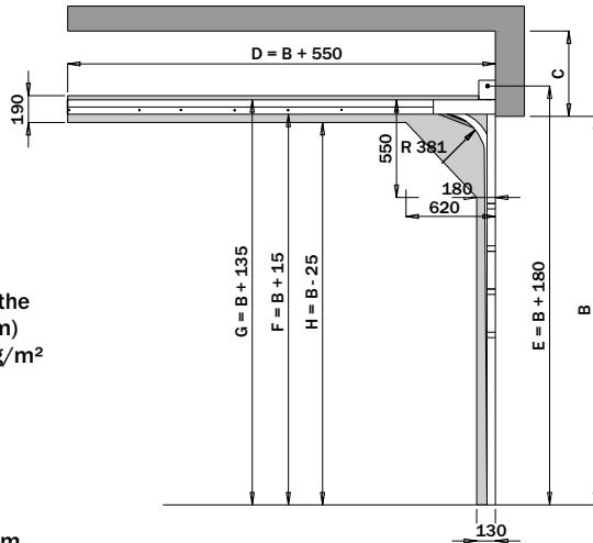
EN A - opening width (from door width 4 950mm there is necessary to add the weight of the struts, number of struts equals the number of the sections, strut weight 1,25 kg/lm)
